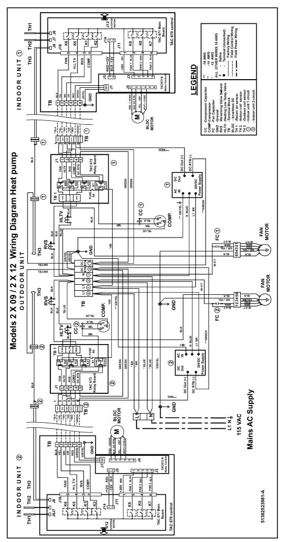
Fig. 13 System Wiring Schematic DFF2HH09J1A, DFF2HH12J1A FAN COIL WITH DFC2H318J2A, DFC2H318J2A Condensing Unit
